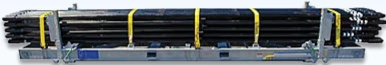
The modular basket includes a self-aligning, interlocking design with folding support stanchions, allowing for up to four empty Pipe Safety Baskets to be stacked for easy transport back to the pipe yard. Five integral retractable ratchet straps and Rumber® pipe stripping material hold the pipe securely in place within the PSB.
