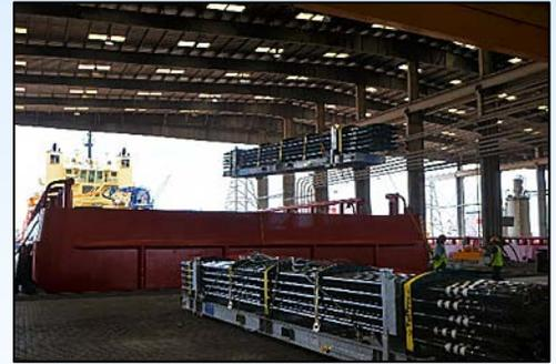
*The patented Knight Oil Tools Pipe Safety Basket takes pipe from the yard to the boat to the pipe deck safely and efficiently. For more info, please view our [PSB Product Highlight Video](#).*
